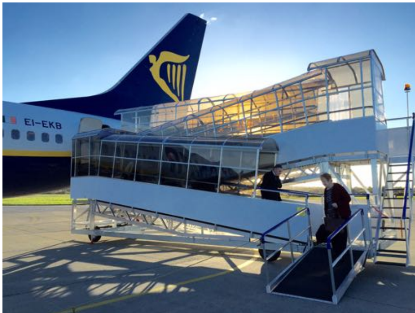
Figure 6-1. Accessible mobile boarding ramp, Kerry Airport, Ireland
